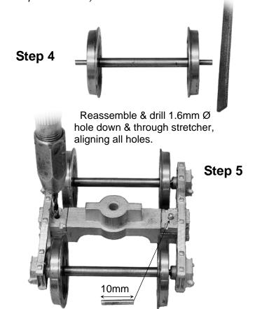
Cut from brass rod & fit assembly pins.
