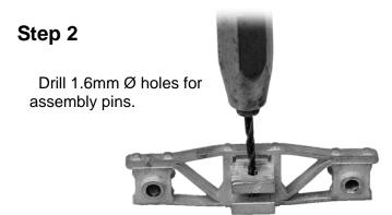
Drill & break through from top and then bottom. Then gently run drill right through to align both holes.
